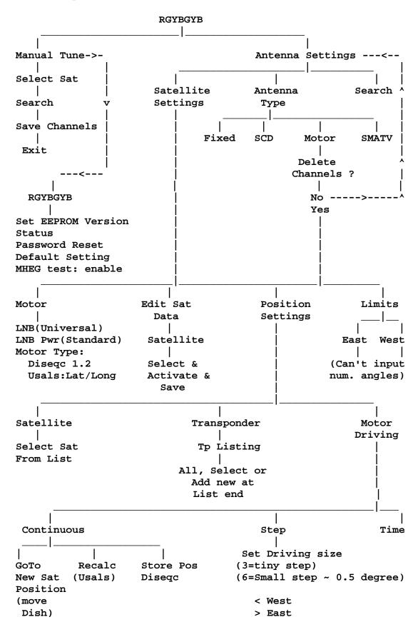
**Set up method using Diseqc 1.2** after normal freesat install with dish at 28.2 east, next enter the hidden menu.
